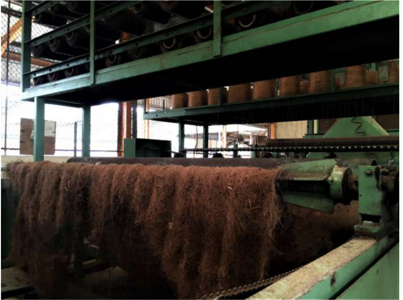
Coconut Fiber Mat Production Equipment in Decommissioned Factory Tikobo 2, Ghana, 2014 Photo Credit: Mae-ling Lokko
